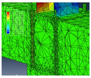
Figure 22. Tensile stress on anchor bolts. Source: [4]
