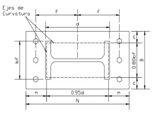
Figure 7. Critical stress zone on the base plate with open core profiles. Source: [12]
