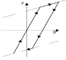
Figure 4. Bilineal model. Source: [4]
