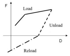
Figure 3. Representation of loading, unloading and recharging phases. Source: [4]
