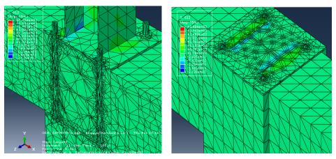
Figure 103. Shear stresses in base plate and anchor bolts. Source: [4]
