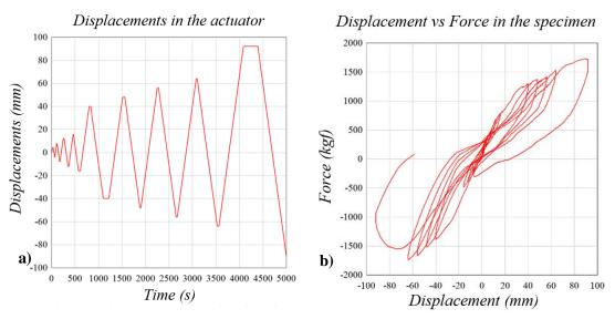
Figure 10. a) Displacement history, b) Concrete cylinders hysteresis. Source: [1]
