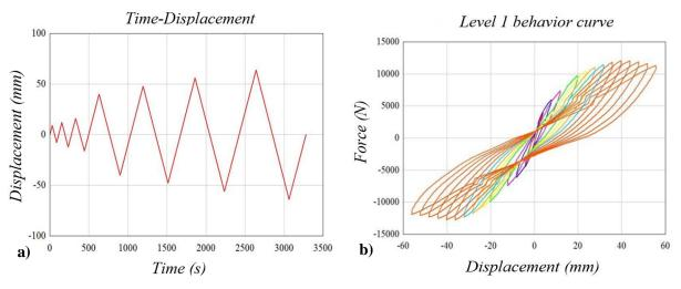
Figure 2. a) A cyclic test example, b) Hysteretic behavior. Source: [1]
