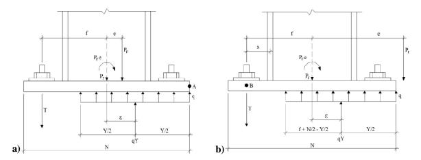
Figure 8. a) Schema of stresses due to small bending moments, b) Large bending moments. Source: [9]
