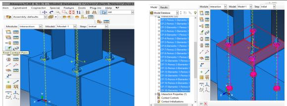
Figure 4. Contact surfaces in the mathematical model. Source: [4]
