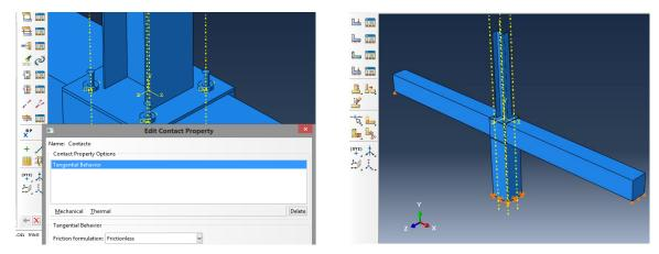
Figure 55. Contact property between surfaces and support conditions for mathematical model. Source: [4]
