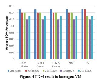
Fig. 4 shown the results of the evaluation with PDM in homogen workload. Based on this figure, it can be seen that the FCM, MMT, and RS methods have the same average yield of 0,13%.
