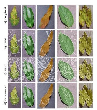
Figure. 5 illustrates examples and correlations with stateof-the-art techniques: (a) Initial image, (b) JSEG technique outcomes, (c) SLIC technique outcomes, and (d) segmented images using the technique proposed
