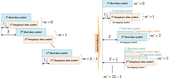
Figure. 2 The overlapping data symbol in FBMC-OQAM system
