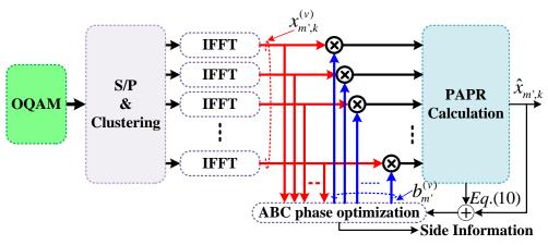
Figure. 3 The block diagram of the proposed PAPR reduction method
