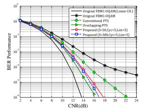
Figure. 8 BER performance for the proposed method in the non-linear channel (IBO=-2dB.)
