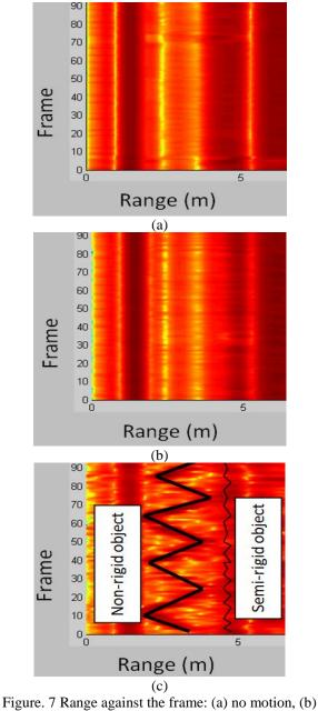
Figure. 7 Range against the frame: (a) no motion, (b) semi-rigid object, and (c) non-rigid body (human), with a semi-rigid object in motion
