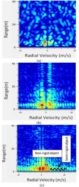
Figure. 6 Range against radial velocity: (a) no motion, (b) semi-rigid object, and (c) non-rigid and semi-rigid
