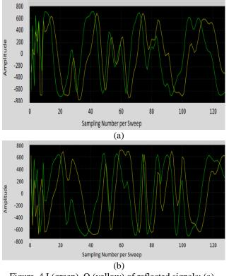
Figure. 4 I (green), Q (yellow) of reflected signals: (a) semi-rigid body and (b) non-rigid body
