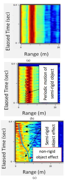
Figure. 5 Elapsed time (sec.) against a range (m): (a) no motion, (b) semi-rigid object in motion, and (c) semirigid and non-rigid objects in motion
