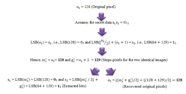
Fig. 2 An illustration of the embedding, extraction, and pixel restoration process for the proposed dual image based modified LSB matching with reversibility technique
