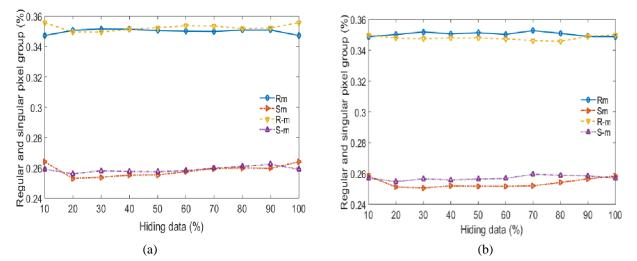
Figure. 5 RS plot for the dual stego-image based modified LSB matching with reversibility technique for: (a) Boat SI 1 and (b) boat SI 2
