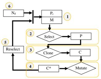
Figure.2 Clonal selection algorithm
