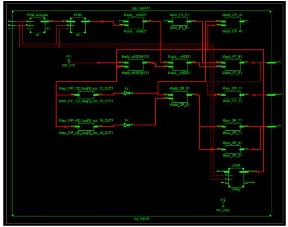
Figure.10 Internal block of the top module for the ID-XT-EA-LFSR algorithm
