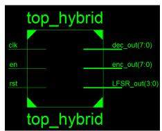
Figure.9 RTL view of the top module for a ID-XT-EA-LFSR algorithm
