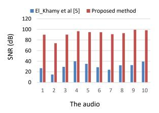
Figure. 4 Results comparison between the proposed method with the previous work after embedding 10 kilobits into each cover file
