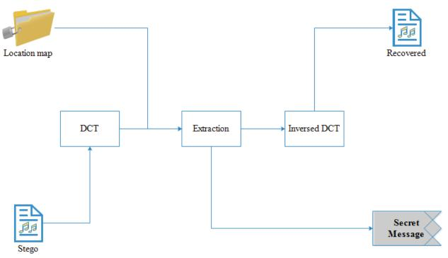
Figure. 2 The extraction procedure
