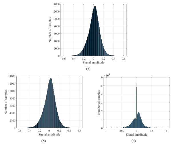
Figure. 6 Audio (No.3) histogram analysis and comparison: (a) original file, (b) stego file using the proposed method, and (c) stego file using El-Khamy et al [5]
