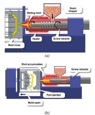
Figure. 1 Injection molding processes: (a) plasticizing the resin and (b) ejecting the work-piece [16]
