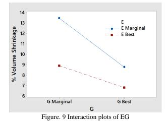
The optimal condition can be set at high level of Packing time (E) and Cooling time (G), which are 6 and 14 seconds, respectively. In Shainin DOE, the setting can yield the lowest volume shrinkage of 5.96 %.
