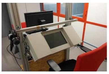
Figure 1. Stationary touch screen mock-up used in this experiment
