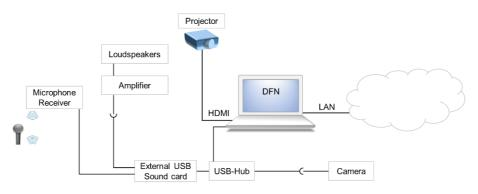
Figure 6. Technology used for broadcasting the lecture
