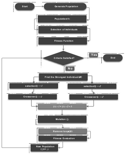
FIG. 2. GENETIC ALGORITHM OPERATORS
