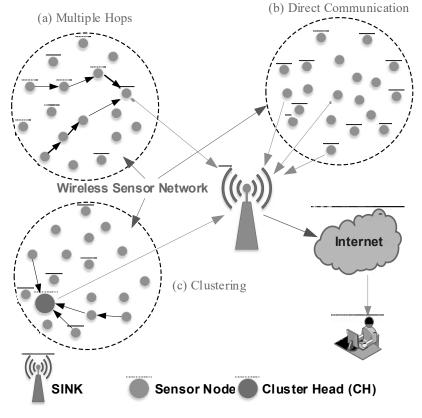
FIG. 1(a). MULTIPLE HOPS, (b) DIRECT COMMUNICATION AND (c) CLUSTERING SCHEMES
