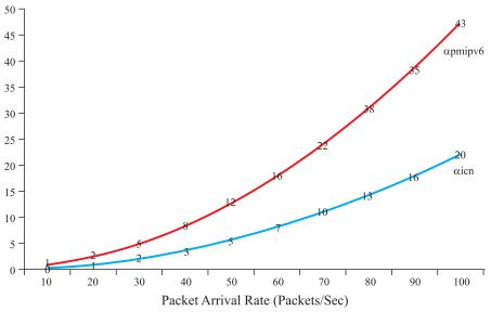
FIG. 5. PACKET LOSS COST FOR ICN AND PMIPV6 VERSUS PACKET ARRIVAL RATE
