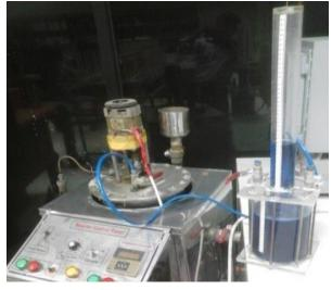
FIG. 2. CSTR WITH METHANE MEASURING JAR
