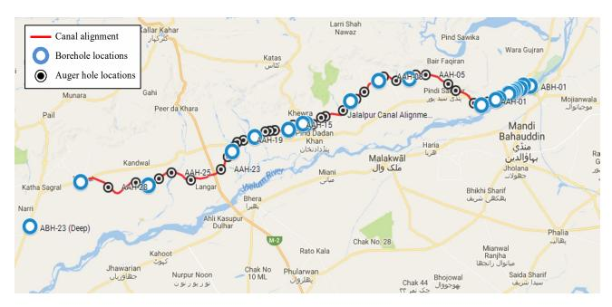
FIG. 1. PROJECT LAYOUT SHOWING BOREHOLE (ABH) AND AUGER HOLE (AAH) LOCATIONS
