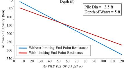
FIG. 5. PILE CAPACITY FOR BORED CONDITION
