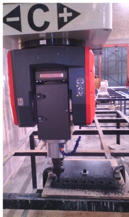
FIG. 1. DRILLING OF HOLES IN THE CFRP COMPOSITE MATERIAL
