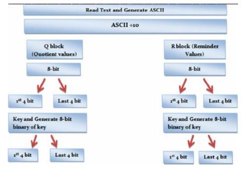
FIG. 4. PROPPSED ALGORITHM FOR ENCRYPTION
