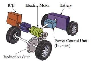
FIG. 5. ILLUSTRATION OF A HEV STRUCTURE [16]
