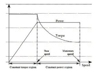
FIG. 1. REQUIRED CHARACTERISTICS FOR EV MOTOR DRIVES [9]
