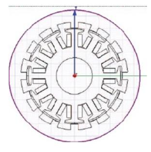
FIG. 8. CROSS SECTION OF PM-SR MACHINE
