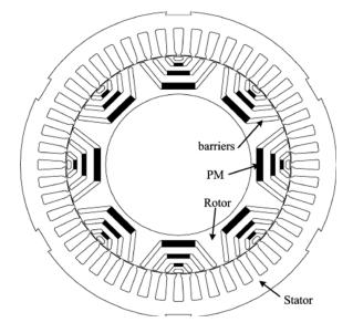
FIG. 7. CROSS SECTION OF PM-ASSISTED SYNCHRONOUS RELUCTANCE MACHINE
