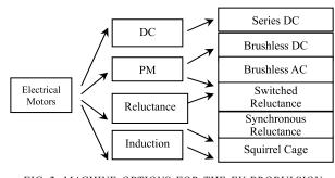
FIG. 2. MACHINE OPTIONS FOR THE EV PROPULSION APPLICATIONS
