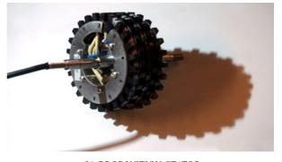
(b) PRODUCTION STATOR FIG. 6 TRANSVERSE FLUX PM MOTOR FOR ELECTRIC BICYCLES [67]
