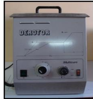
Fig. 5: Controlled water bath
