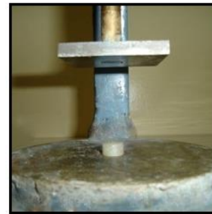
Fig. 6: Sample placed under the axial load of vicat apparatus
