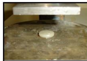
Fig. 7: Sample after applying axial load 40^\circ\text{C} and 45^\circ\text{C} from right to left side
