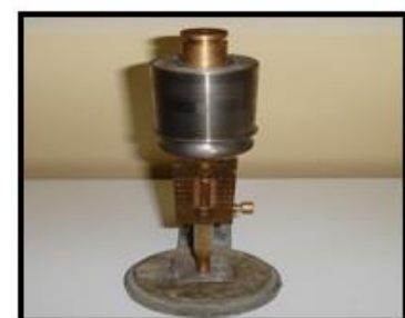
Fig 2: Vicat apparatus after modification
