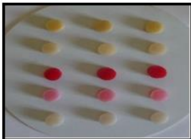
Fig. 4: Samples of different waxes used in flow, hardness and accuracy test
