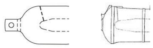
Fig. 32. Breech and chamber of Dahlgren 9in SB
