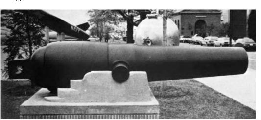
small powder charges in the Palliser conversions, which relied on the cast iron of the original gun to support the low steel inserted tube.
