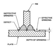
Fig. 3 Geometrical aspects related to toe grinding process [15]
