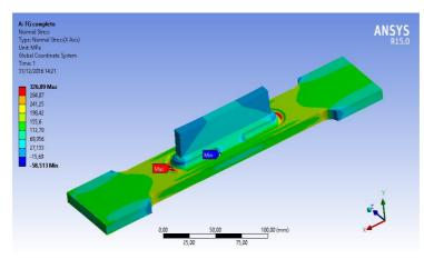
Fig. 12 Obtained results for the case of contour groove at the rib tip
