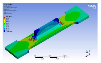
Fig. 13 Obtained results for the case of a straight groove at the rib tip.
