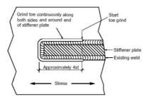
Fig. 5 Recommended contouring toe-grinding [11]
