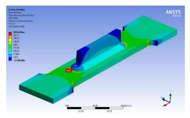
Fig. 11 Post-processing image obtained for the no-grinding case.
