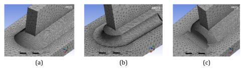
Fig. 9 Resulting meshes: a) without toe grinding, b) with a contouring toe grinding and c) with straight toe grinding.
