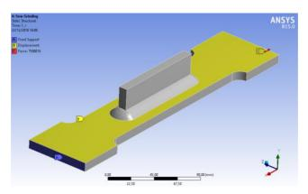
Fig. 10 Boundary conditions taking the no-grinding specimen as an example.
