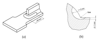
Fig. 7 Groove geometry of the second study case: a) overall geometry and b) cross cut of the groove.
