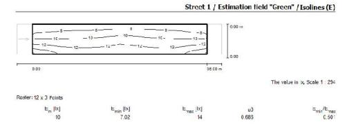
Figure 3. Lighting indicator values and isolux curves.
