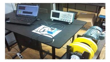
Figure 2. Experimental arrangement for acquisition, monitoring and vibration analysis at an induction motor.
