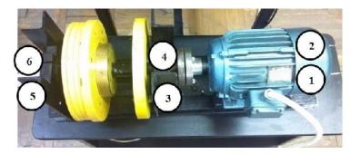
Figure 3. Vibrations measurement points.
