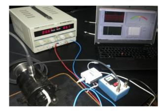
Figure 11. Experimental arrangement for acquisition, monitoring and vibration analysis at a micro DC motor.
