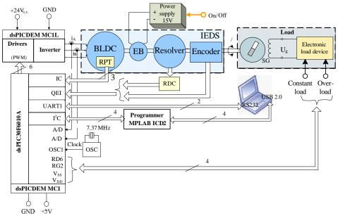
Figure 1. EDS block diagram.
