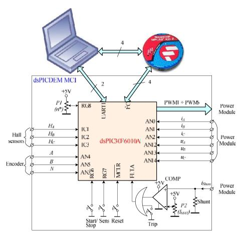
Figure 2. dsPICDEM MC1 development system block diagram.
