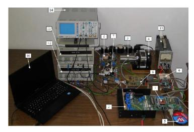
Figure 7. General view of the test bench: 1–development system, 2–power module, 3–IEDS, 4–SG, 5–MPLAB ICD2 programmer/debugger, 6–current transducers interface, 7–voltage transducers interface, 8–RDC, 9–electronic load device, 10–PC, 11, 12, 13–power supplies, 14–osciloscope.
