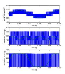
Figure 2. The output phase voltage of the three-phase power inverter and the fundamental signal, insertion of the third harmonic order based on the eq.22. and the modulating signal
