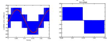
Figure 3. Phase output voltage and the fundamental and the line output voltage
