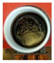
Figure 7. The movement spectrum for the use of a magnetoactive particles slurry for GROSU – CERNOMAZU motor, according to the phase sequence [15]: a). Direct sequence (R-S-T); b). Reverse sequence (T-S-R)
