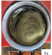
Figure 4. The movement spectrum for the use of a magnetoactive particles slurry, according to the phase sequence [42]: a). Direct sequence (R-S-T); b). Reverse sequence (T-S-R).
