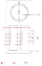
Figure 1. GROSU three – phase motor [67, 68, 69, 70, 71]: 1 - stator; 2 – phase windings; 3 – cage armature.
