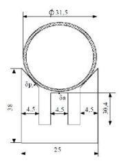
Figure 3. Dimensions of the magnetic core of the GROSU motor stator used in the experiments [42].
