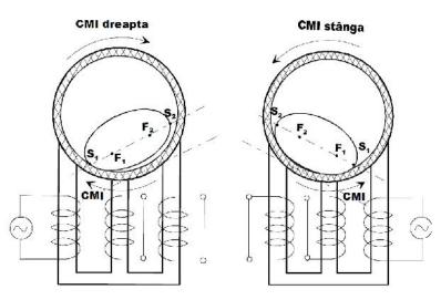
Figure 6. GROSU-CERNOMAZU motor. The ferrofluid movement spectrum has the shape of a distorted ellipse, with the major axis oriented in the shielded pole direction [15].
