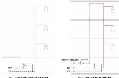
a) without recirculation b) with recirculation **Figure 1.** Plumbing installation for domestic hot water supply
