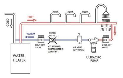
Figure 6. Recirculation pump which requires recirculation pipe [12]
