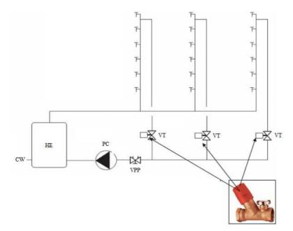
**Figure 4.** DHW plumbing installation with recirculation, heat exchanger, recirculation pump, valves with pressure inlet and thermostatic taps [2]
