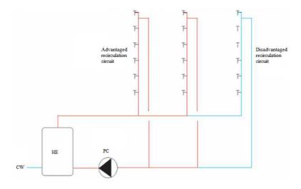
**Figure 2.** DHW plumbing installation with recirculation, heat exchanger and recirculation pump [2]
