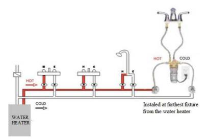
Figure 5. Recirculation pump without recirculation pipe [12]
