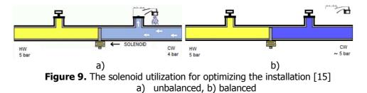
As it is shown in Figure 9, the advantage of using this solenoid is the installation hydraulic balancing [15].
