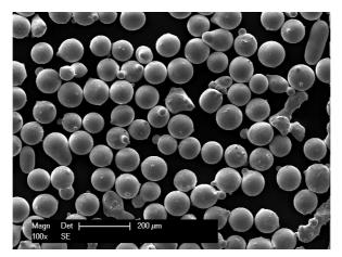
Figure 1. SEM-micrograph of the NiCrBSi powder
