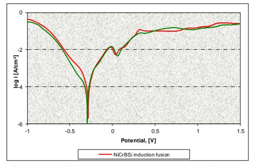
Figure 4. Potentiodynamic polarization curves of the samples tested in a 3,5% NaCl solution
