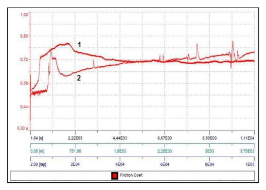
**Figure 5.** Sliding wear friction coefficients of the tested coatings: induction fused (1) respectively flame fused (2)
