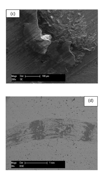
**Figure 6.** SEM-micrographs of the worn surface of the induction fused coating (a, b) respectively of the flame fused coating (c, d)
