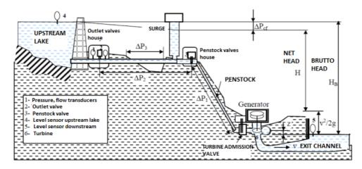
Figure 5. Measurement and drive systems on the hydraulic circuit of the power plant
