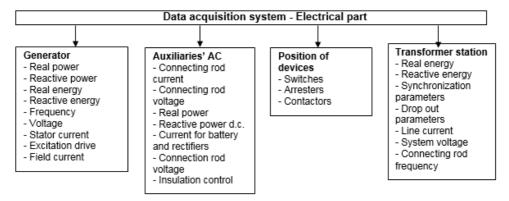
Figure 4. Data acquisition system – Electrical part
