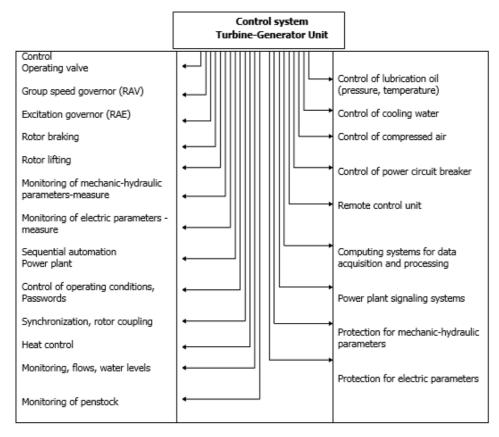
Figure 1. Control systems for hydropower groups
