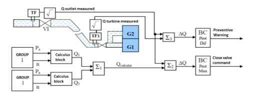
Figure 6. Maximal and differential protection at penstock breakage
