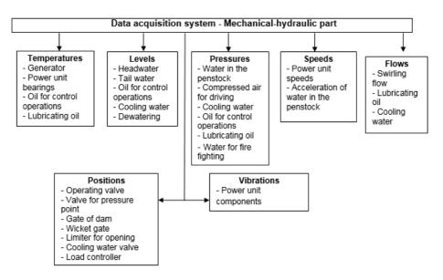
Figure 3. Data acquisition system - Mechanical-hydraulic part
