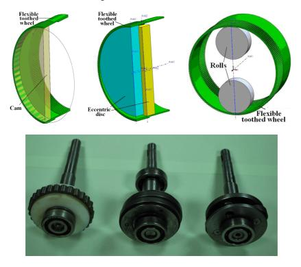
Figure 2. The models of a waves generator.
