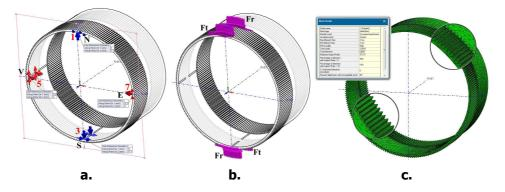
Figure 3. Restrictions applied the tasks and meshing to the flexible wheel.
