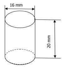
Figure 1. Schematic representation of the aluminum specimens
