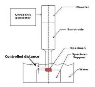
Figure 2. The principle of the indirect cavitation method
