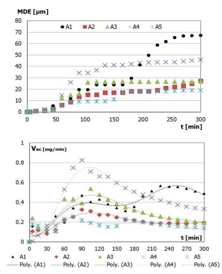
Figure 4. The variation of the cavitation erosion rate for all specimens
