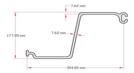
Figure5. Pile plank vinyl polychloride
