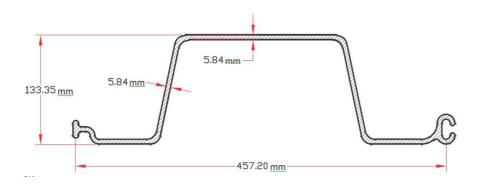
Figure2. Pile plank vinyl polychloride
