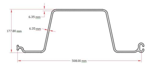
Figure 3. Pile plank vinyl polychloride
