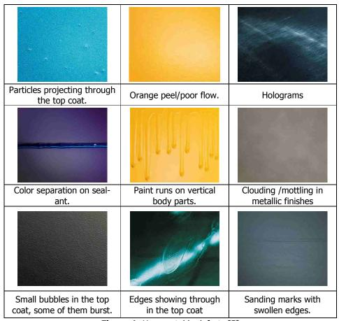
Figure 1. Unacceptable defects [5]
