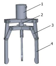
Figure 1. The model of robotic gripper.
