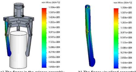
a) The finger in the gripper assembly b) The finger visualized separately **Figure 8.** Coloured map of von Mises stress.
