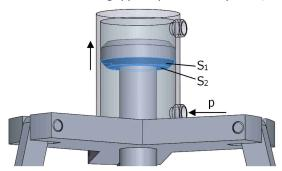
Figure 4. Gripper's pneumatic cylinder.
