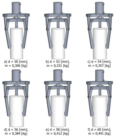
**Figure 3.** Cylindrical workpieces of the same length, but with different diameters, grasped by the gripper.
