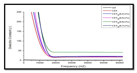
Figure 2: Electrical insulation constant as a function of frequency of carbon fiber epoxy composites and alumina nanoparticles with different weight ratios.
