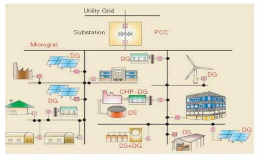
Figure 1: The general form of a microgrid (Katiraei, 2008)
