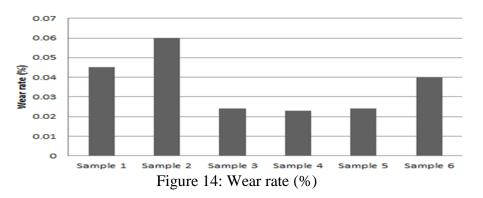
When the wear rate graph shows that the maximum material loss is sample 2 samp. 1, samp. 6 samp. 3, samp. 5 and samp. 4 It can be seen.
