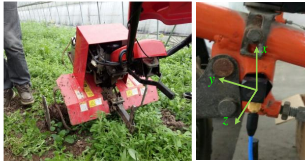
Fig. 1 - Electric elementary prototype and battery box
