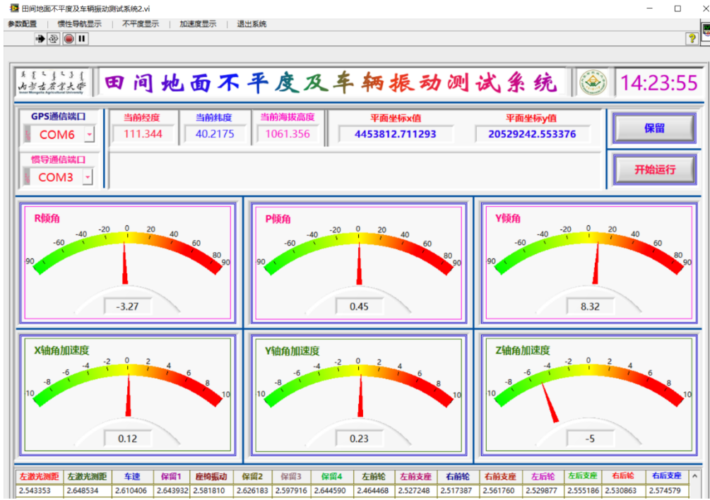
Fig. 3 – Software interface of profiling data acquisition system
