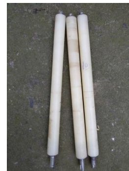
Fig. 5 - Physical drawing of separating rollers
