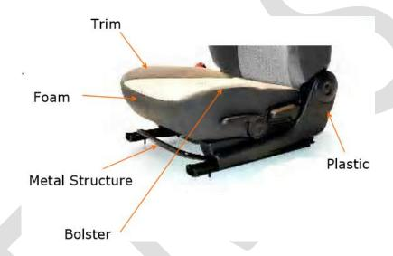
Seat cushion is important in order to get the thighs support and position of occupants. During the manufacturing of seat cushions polyethers are used.
