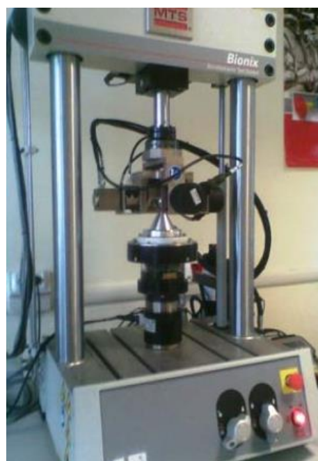
Fig. 2. MTS Bionix servo-hydraulic multiaxial dynamic testing machine, equipped with system for testing the hip implants.
