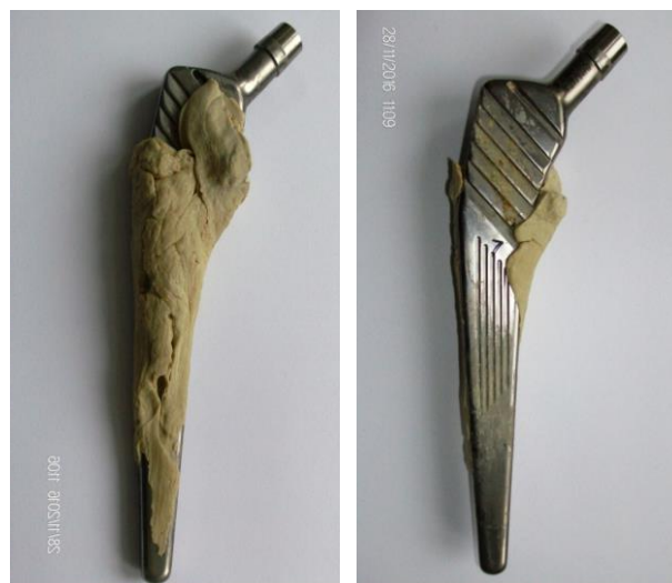
Fig. 10. The sides of the cemented stem prosthesis together with a part of the cement mantle, extracted after 2450000 cycles of fatigue test, from Instron® device.
