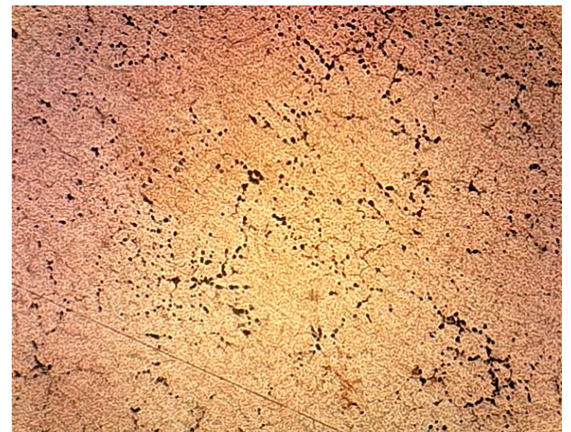
Fig. 8. Optical micrograph of MMC at 8 % reinforcement and 80 mesh size.
