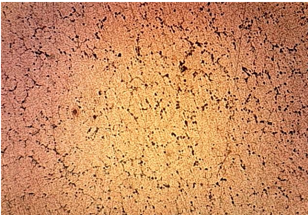
Fig. 10. Optical micrograph of MMC at 16 % reinforcement and 200 mesh size.
