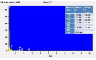
**Fig. 10.** Energy dispersive X-ray analysis (EDXA) of NCD Coatings.
