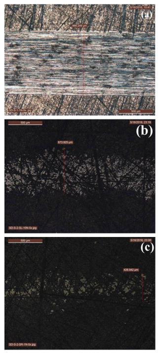
**Fig. 7.** Images of wear track of CVD-diamond coatings, (a) surface morphology of virgin substrate, (b) Surface morphology of NCD coatings, (c) Surface morphology of MCD coatings.
