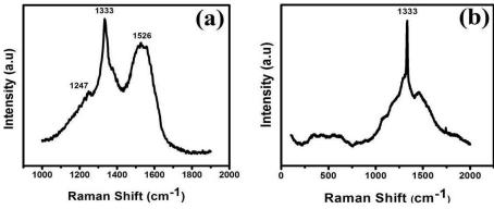
Fig. 2. Raman spectra of CVD-diamond coatings, (a) NCD and (b) MCD.
