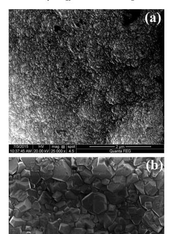
**Fig. 1.** CVD-diamond coatings, (a) Surface morphology of NCD coatings, (b) Surface morphology of MCD coatings.
