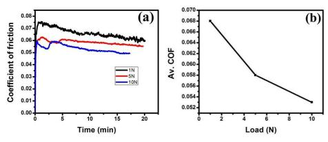
**Fig. 6.** Tribological characteristics of NCD coatings sliding against alumina ball, (a) Coefficient of friction vs duration of rubbing at 1 N, 5 N and 10 N, (b) Average coefficient of friction vs. normal load.
