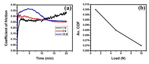
**Fig. 5.** Tribological characteristics of MCD coatings sliding against alumina ball. (a) Coefficient of friction vs duration of rubbing at 1 N, 5 N and 10 N, (b) Average coefficient of friction vs. normal load.
