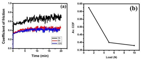
**Fig. 4.** Tribological characteristics of Ti6Al4V substrates sliding against alumina ball. (a) Coefficient of friction vs duration of rubbing at 1 N, 5 N and 10 N, (b) Average coefficient of friction vs. normal load.
