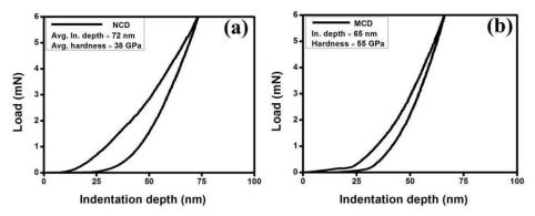
Fig. 3. (a) Load-displacement curve for NCD coating, (b) Load-displacement curve for MCD coating.
