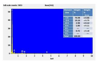
**Fig. 9.** Energy dispersive X-ray analysis (EDXA) of MCD Coatings.
