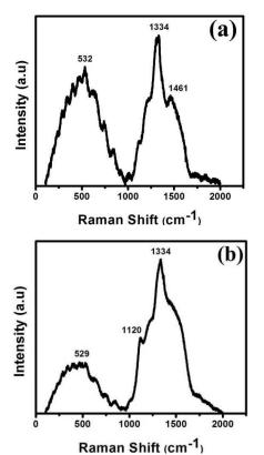
**Fig. 8.** Raman spectra of wear track of CVD-diamond coatings, (a) NCD and (b) MCD.
