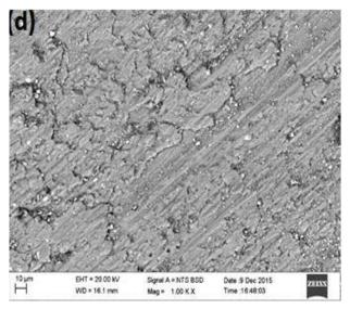
Fig. 3. Worn out surface analysis at various conditions a) L = 10N, V = 1m/s, S.D = 400m b) L = 10N, V = 2m/s, S.D = 800m c) L = 10N, V = 4m/s, S.D = 1600m d) L = 30N, V = 1m/s, S.D = 1200m.
