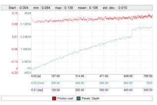
**Fig. 7.** Friction force and penetration depth dependence on time/sliding distance/laps for ZA-27 nanocomposite reinforced with 1 vol. % Al2O3, obtained under 200 mN normal load and 2 mm/s sliding distance [9].
