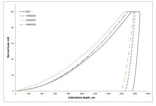
**Fig. 5.** Nanoindentation curves for ZA-27 alloy and tested nanocomposites reinforced with 1, 3 and 5 vol. % of Al<sub>2</sub>O<sub>3</sub> [9].
