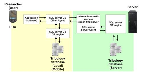
Fig. 11. Replication architecture.
