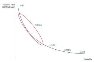
**Fig. 3.** Relationship between transfer rate and mobility technologies for data transfer.
