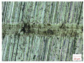
**Fig. 8.** Optical microscopy of wear tracks for ZA-27 nanocomposite reinforced with 1 vol. % Al<sub>2</sub>O<sub>3</sub>, obtained under 200 mN normal load and 2 mm/s sliding distance [10].
