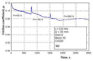
**Fig. 4.** Change the coefficient of friction in oil samples SU.
