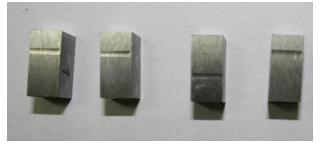
Fig. 7. Wear scar on the blocks in tribological tests.
