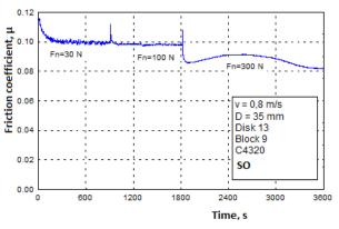
Fig. 3. Change the coefficient of friction in oil samples SO.
