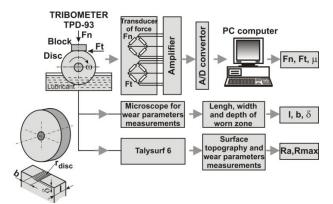
**Fig. 1.** Measuring system for the determination of wear characteristics.
