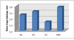
Fig. 6. Measured width of the scar wear on block.
