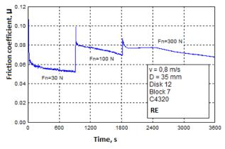
Fig. 2. Change the coefficient of friction in oil samples RE.
