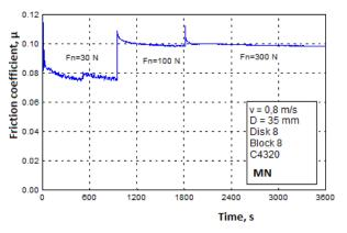
**Fig. 5.** Change the coefficient of friction in oil samples MN.
