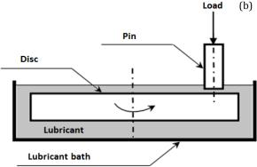
**Fig. 1.** (a) General view of the tribometer and (b) pinon-disc configuration.
