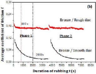
**Fig. 3.** Evolution of the average coefficient of friction versus duration of rubbing: (a) brass/steel and (b) bronze/steel.
