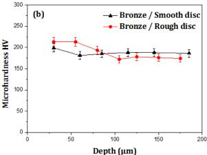
**Fig. 6.** A variation of the microhardness of subsurface layers versus a depth of: (a) Brass and (b) bronze samples after friction.
