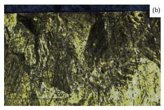
**Fig. 5.** Microscopic image of an orthogonal cutting to the track of wear after friction of: (a) brass and (b) bronze.
