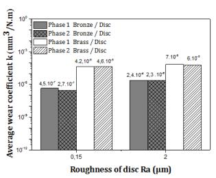
**Fig. 4.** Average wear coefficient of brass and bronze pins versus disc surface roughness ( $Ra = 0.15 \mu m$ ,  $Ra = 2 \mu m$ ).
