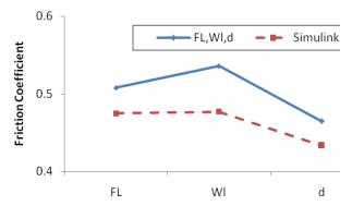
**Fig. 13.** Comparison of friction coefficient from equations and simulink brake model.
