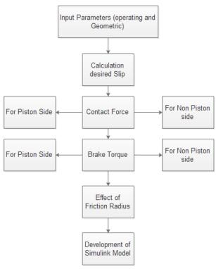
**Fig. 10.** Algorithm for friction coefficient estimation.
