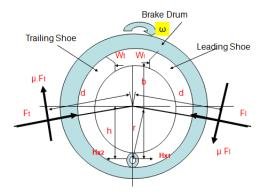
**Fig. 2.** Equillibrium diagram for the drum brake when contact force is inclined.
