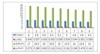
Fig. 19. Comparison of friction coefficient  $(\mu)$  with friction radius.
