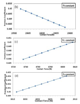
**Fig. 16 (a-d).** Friction Coefficient profiles for variations in contact force for disc brake.
