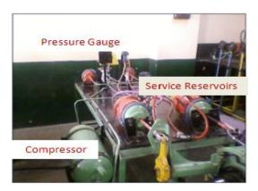
Fig. 8. Braking System set up.
