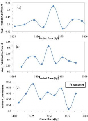
**Fig. 15(a-d).** Friction Coefficient profiles for variations in contact force for drum brake.
