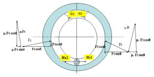
**Fig. 3** Force analysis for both the shoes of the drum brake.
