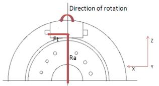
Fig. 6. Tangential force at the calliper.
