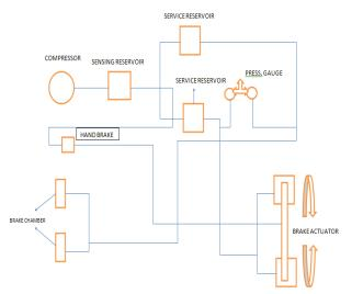
Fig. 7. The layout of Braking System set up.
